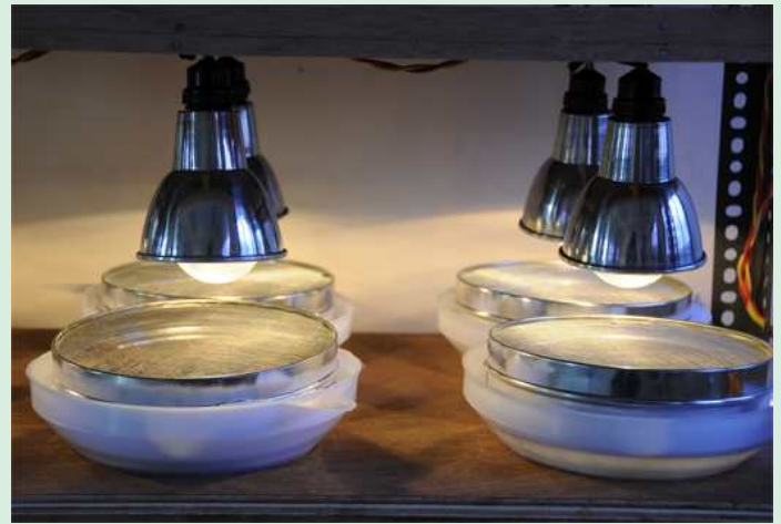
Modified Burlese Funnel for extraction of soil arthropods
