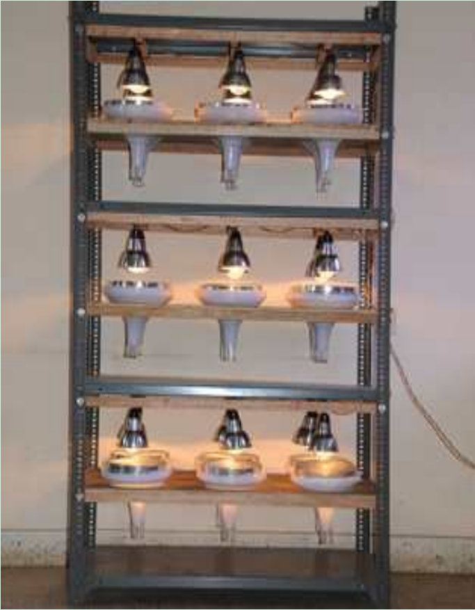
Modified Burlese Funnel for extraction of soil arthropods
