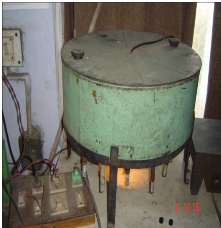
Fig. M2. Exterior view of the Tullgren Funnel extraction Apparatus.
