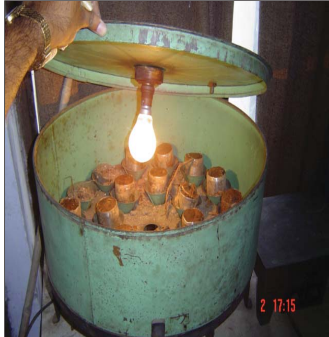
Fig. M2a. Extraction of soil arthropods by a Tullgren extraction apparatus modified by Macfadyen.
